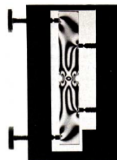
Photoelastic fringes in a notched beam loaded in bending.
