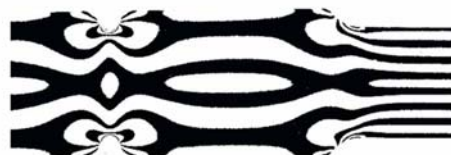
Photoelastic fringes in a notched beam loaded in bending.
